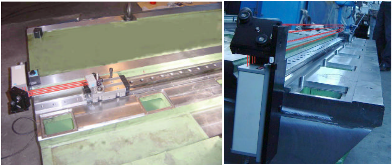
Horizontal straightness measurement (left) and Vertical straightness measurement (right) on a roller guide mounted on a machine tool basement. Measures performed with Optodyne Dual Beam laser Doppler Displacement Meter.
