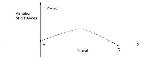
Fig. 1 Measurement of parallelism of two guide ways by a LDDM dual-beam laser system
