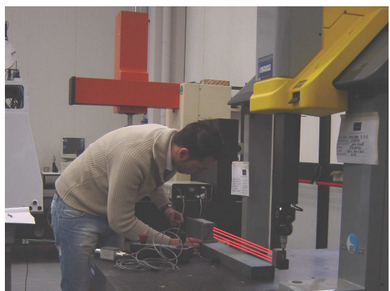
Simultaneous: Positioning, Pitch angle, and Straightness on CMM with MCV2002
