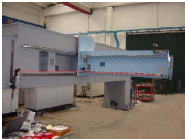
Fig. 5 Squareness measurement on a large machine tool, the laser head on he left, the pentaprisim in the center and the quad detector on the right
