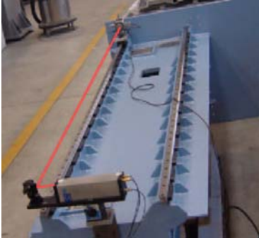
Fig. 3 Mounting and Alignment of quidway
